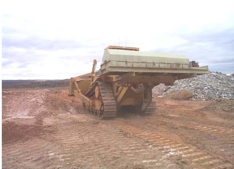
Figure 3: Winged tines on Cat D8
